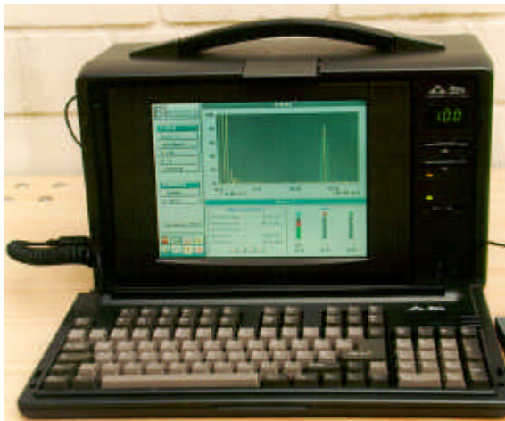
Fig.2: Portable PC used as ultrasonic system
