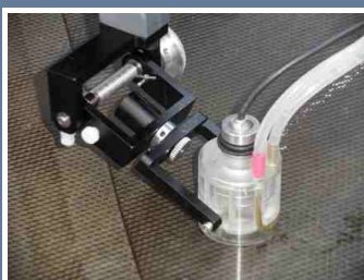
Cardanic fixed transducer adapter with built-in focal immersion transducer
