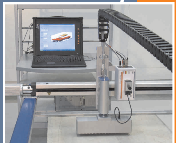
Components of Flexus Concrete : ultrasonic system, transducer array, multiplexer, and scanner with controller
