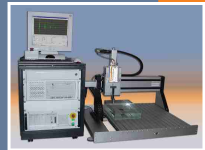
Pulser/ receiver unit mounted at the scanner
